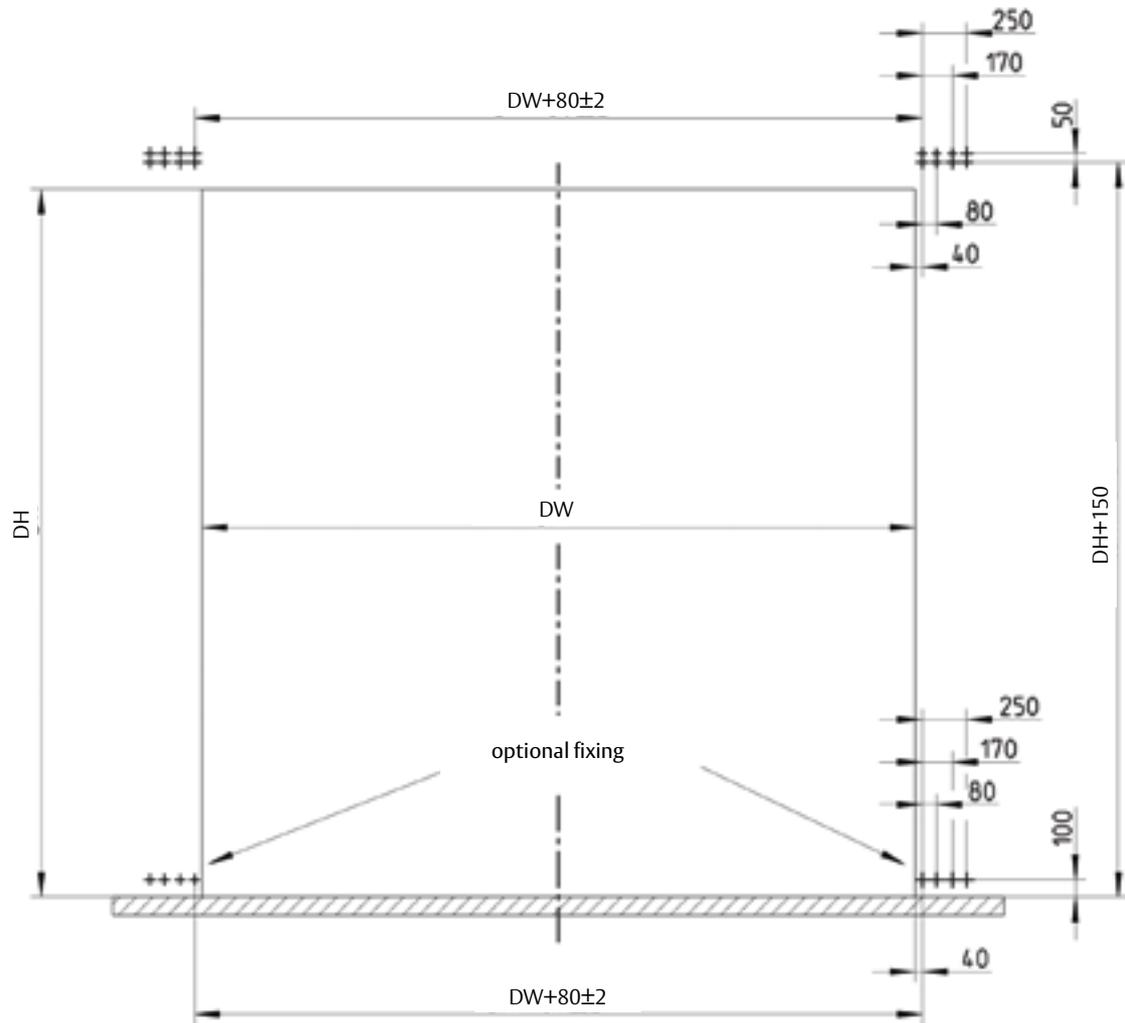
Fixing screws M12 or comparables
